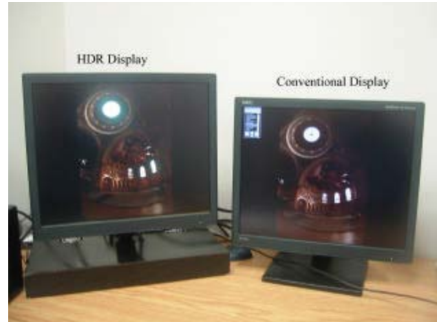
High Dynamic Range Display (left) next to comparable conventional display (right). Notice high brightness bloom in the top window of the Stanford Memorial Church image.
